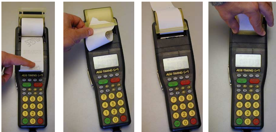
feed the paper through the paper opening
